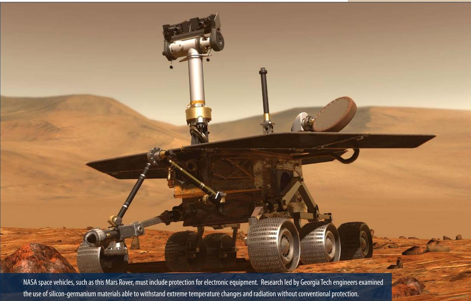
NASA space vehicles, such as this Mars Rover, must include protection for electronic equipment. Research led by Georgia Tech engineers examined the use of silicon-germanium materials able to withstand extreme temperature changes and radiation without conventional protection.
